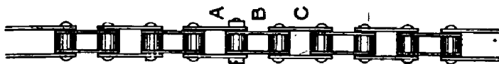
FIG. 4.—The junction portion of a roller chain which requires shortening by one link.
