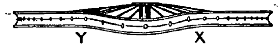
FIG. 1.—Showing a wheel which has had the tyre bent out of truth from the point X to the point Y.
