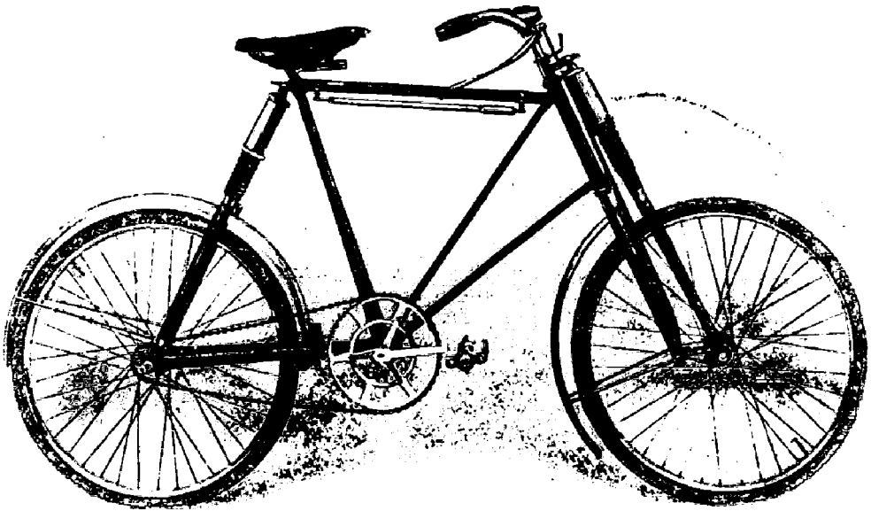
A CYCLE FITTED WITH SHARP AIR-SPRINGS BEHIND THE SADDLE AND ON THE FRONT SPRING-FORK.
