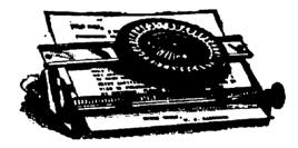
This is a very complete machine, having key for each letter, roller feed, automatic inking and spacing, sight writing. Will take a small letter head, and can be easily and rapidly operated. By reversing the carriage the machine can be used for addressing packages or writing in books. Has feed roller as shown.
