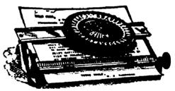
This is a very complete machine, having key for each letter, roller feed, automatic inking and spacing, sight writing. Will take a small letter head, and can be easily and rapidly operated. By reversing the carriage the machine can be used for addressing packages or writing in books. Has feed roller as shown.
