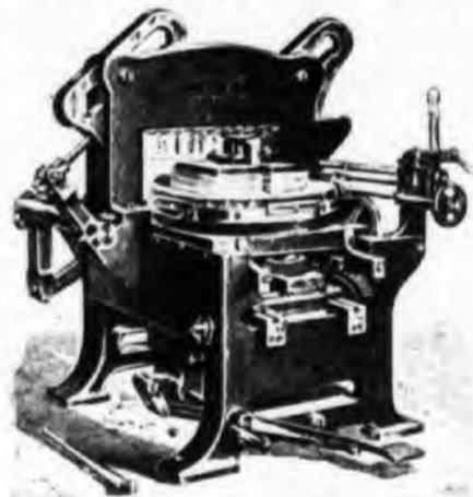
DOUBLE THREE-SIDED TRIMMER for cutting or trimming TWO piles of folded paper and books ON ALL EDGES with ONE SINGLE CLAMPING.
