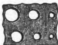
This illustration shows the actual size of holes that may be cut with the leather punch blade.
